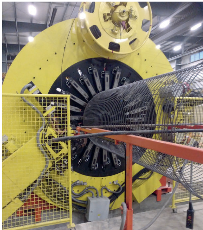
A rotating welding head combined with another coil ensures that one cage after another can be produced continuously.
