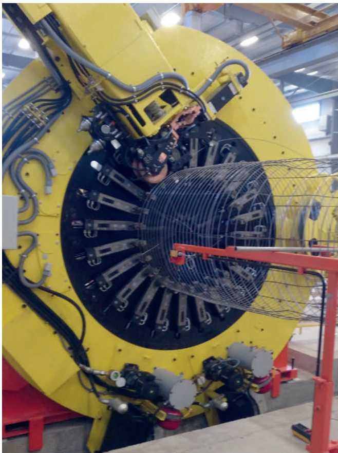
apilion ASMS with 24 longitudinal wires and automatic cutting device
