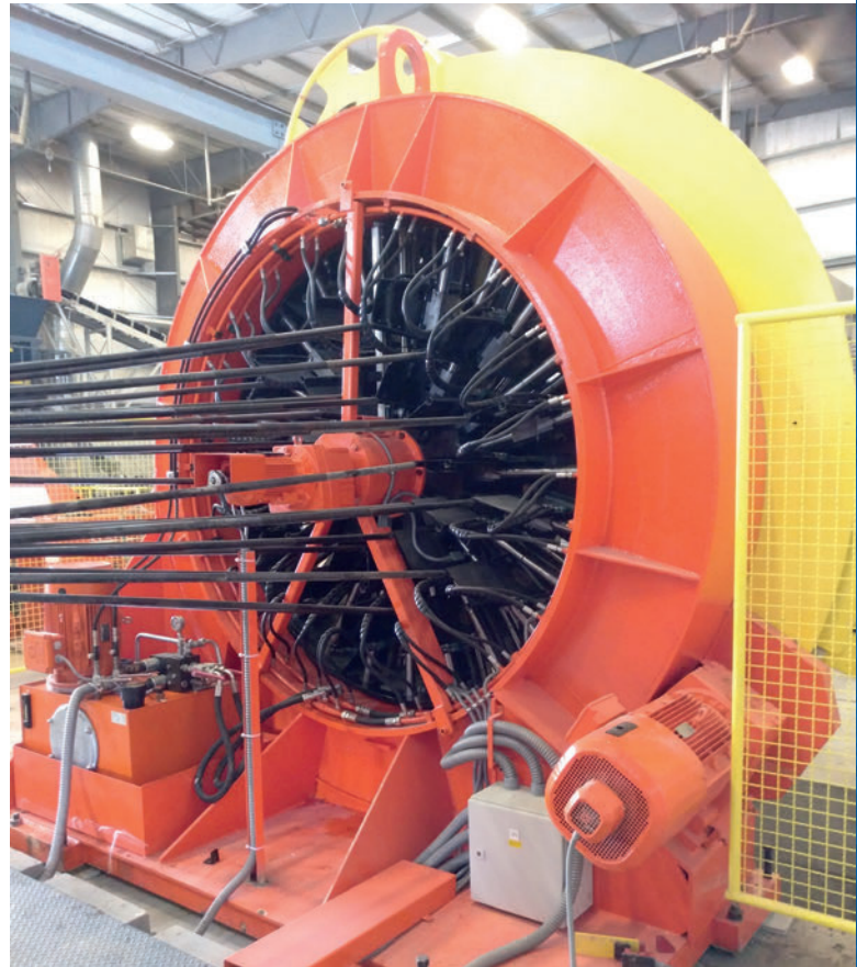
The longitudinal wires are unwound from coils and fed fully automatically into the machine.
