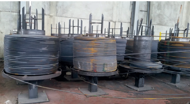
Longitudinal wires with diameter 18mm wound on 3to spools
